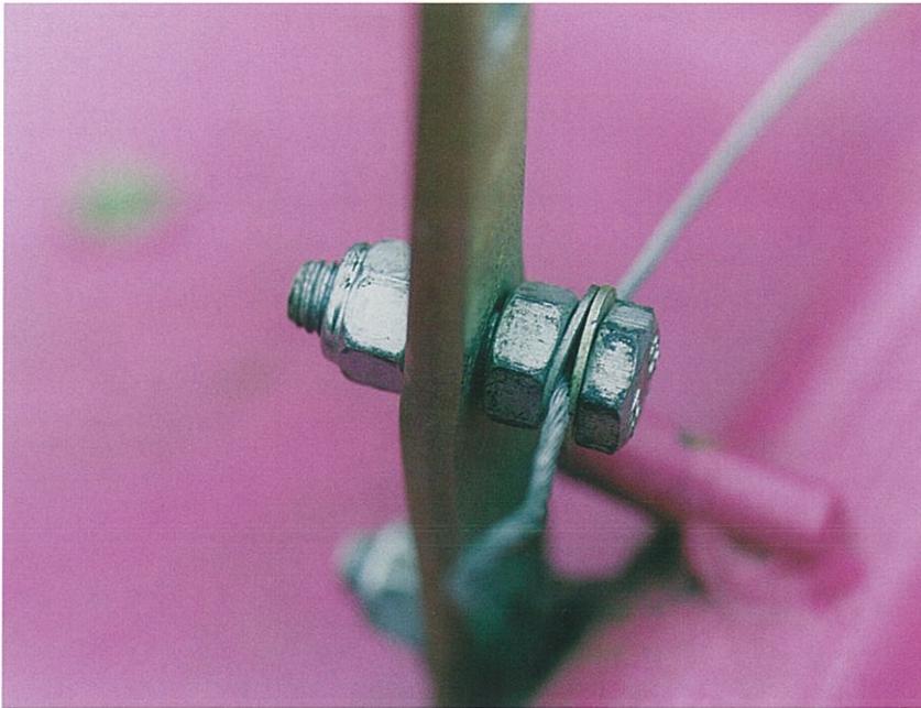
Fig. 8.8. The cable is fixed to the pedal using a bolt, two washers and two nuts. The nut holding the cable should be tight, but the other should be left slightly loose to allow the bolt to rotate. (Steve Williams)
