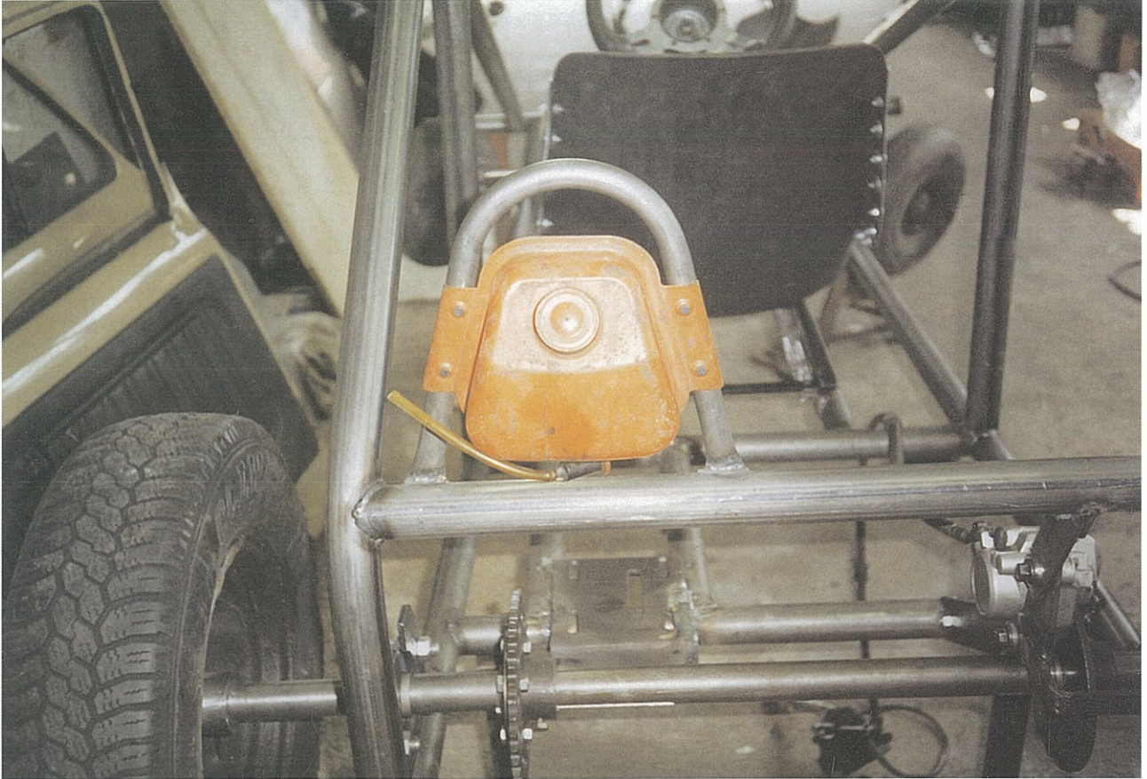
Fig. 6.2. An alternative type of lawnmower fuel tank mounted on a bent tube welded to the Buggy frame. (Derek Manders)
