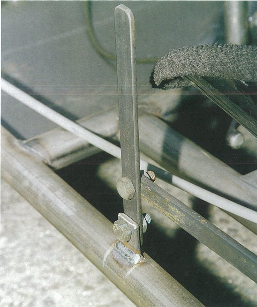
Fig. 8.15. The gear-change lever assembly in position on the Buggy frame. (Steve Williams)
