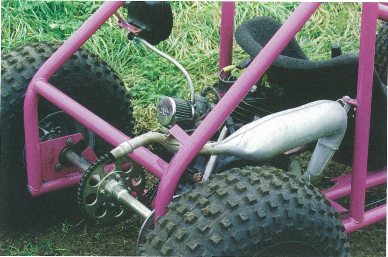
Fig. 6.4. On the original Buggy two brackets were welded to the frame to mount the exhaust. (Steve Williams)
