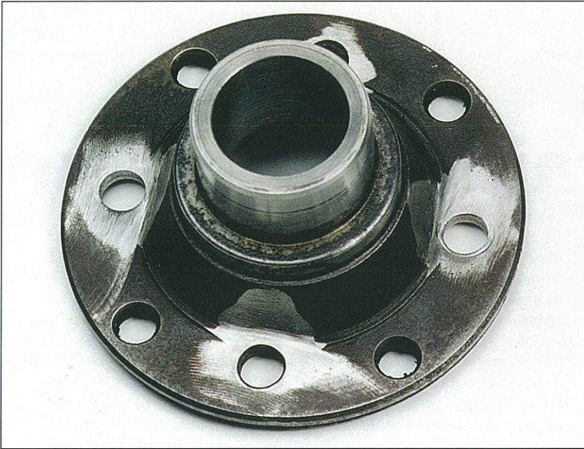
Fig. 7.2. The Ford rear differential flanges will need to be machined to suit the rear axle, sprocket, brake disc and wheels you are going to use. (Steve Williams)
