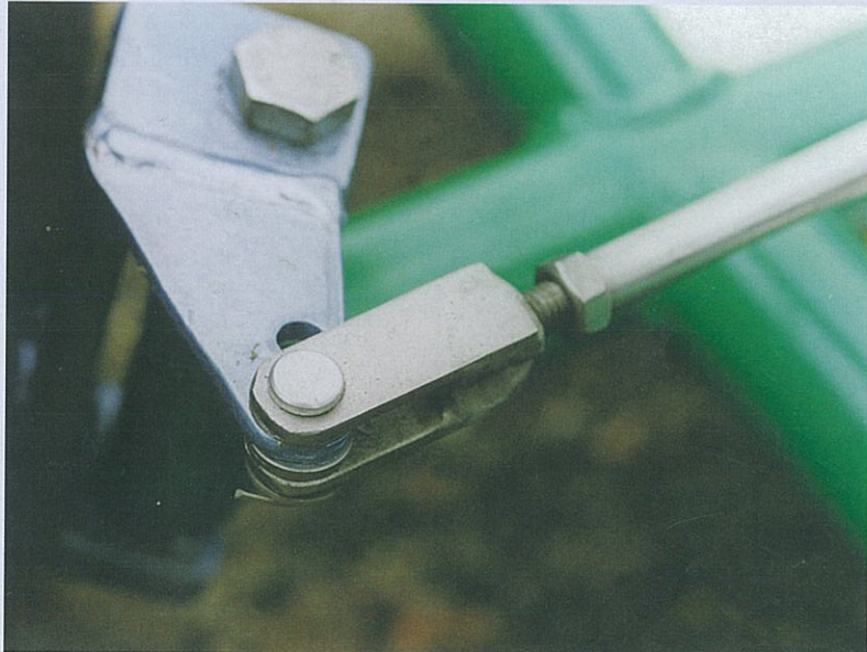
DIY track-rod end connected to steering arm using a clevis-pin and split-pin. (Steve Williams)
