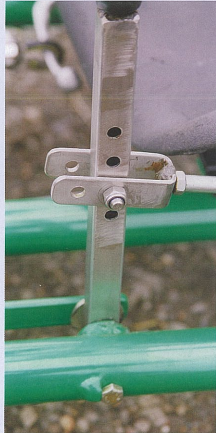
An alternative design of gear-change lever made from box-section steel. (Steve Williams)
