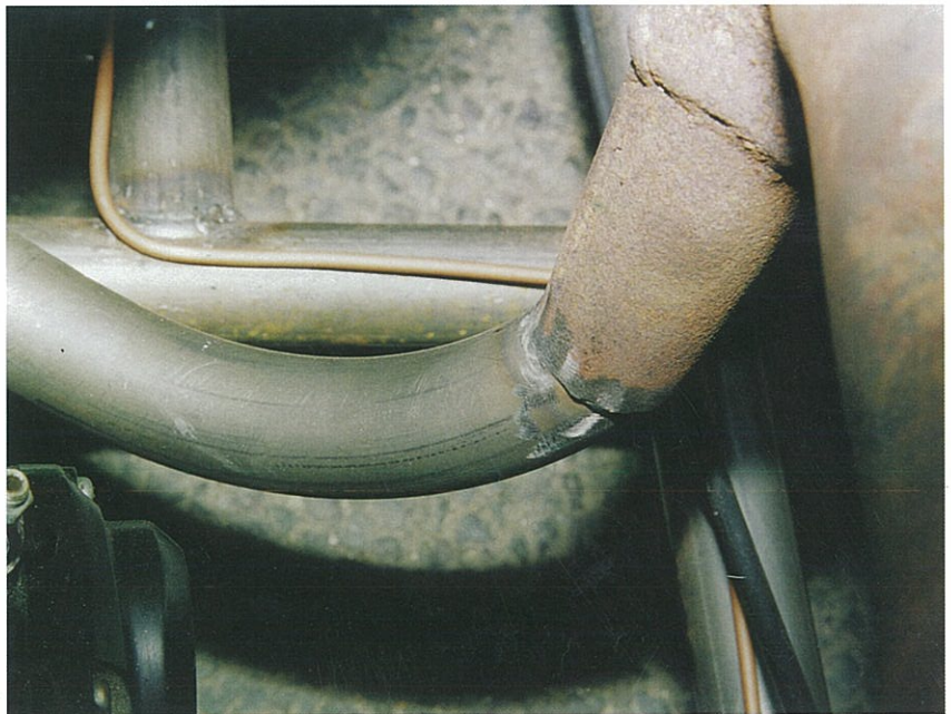
Fig. 6.3. The exhaust was cut, rotated and re-welded so it exited at the back of the buggy. We were careful not to change the length or volume of the exhaust. (Steve Williams)
