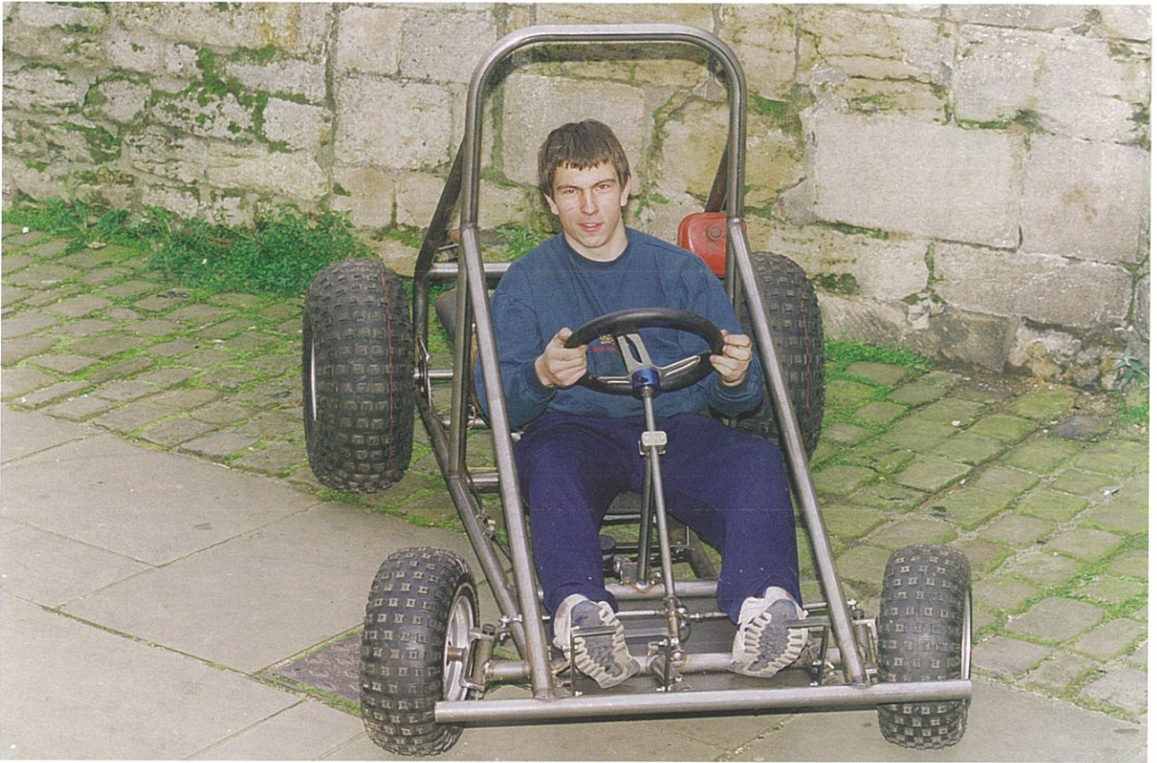
Fig. 9.2. A final check to make sure everything is in the right place. It's better to make any changes now rather than to have to do more drilling and welding after your Buggy has been finished. (Steve Williams)
