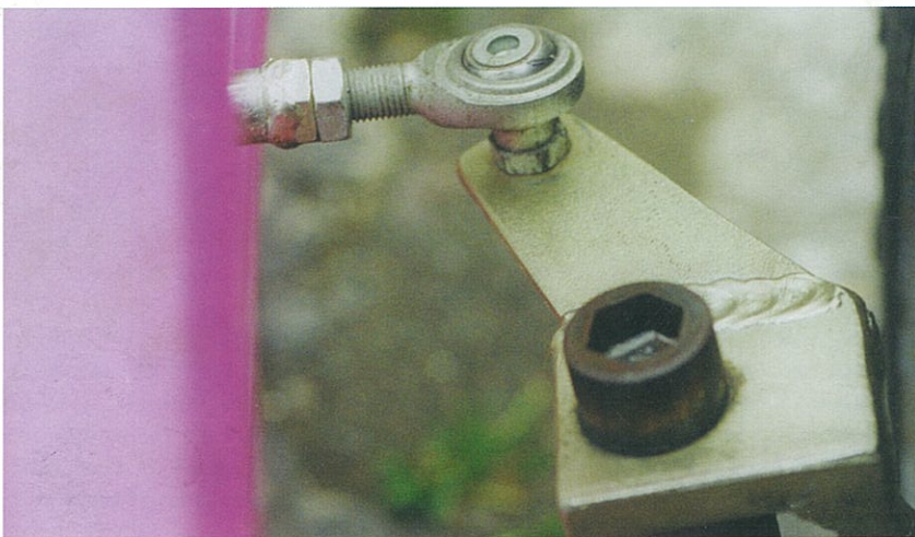
Fig. 5.19. On the original Buggy, the track-rod ends have threaded pins which are secured to the steering arms by Nyloc nuts. (Paul Buckland)
