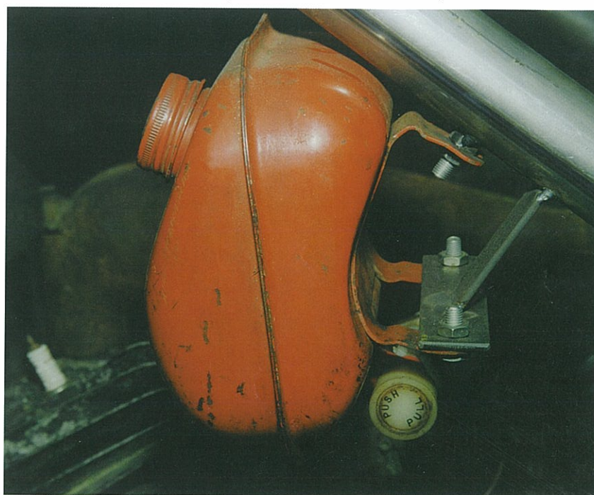
Fig. 6.1. The petrol tank on the original Buggy, showing the simple bracket made to fix it in position on the frame tube. Note also the bolt which secures the tank's top bracket. (Steve Williams)
