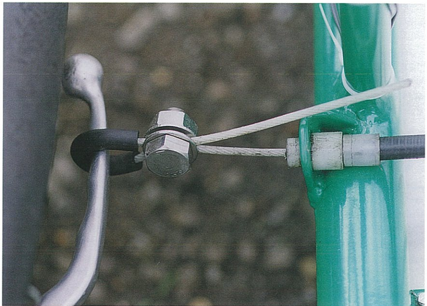
Fig. 8.7. An alternative method of fixing the brake operating cable to the hand-brake lever. (Derek Manders)
