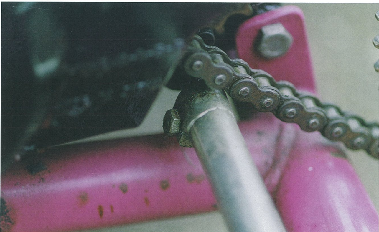
Fig. 8.14. Gear-change tube splined boss fitted over the end of the gearbox splined shaft. (Steve Williams)
