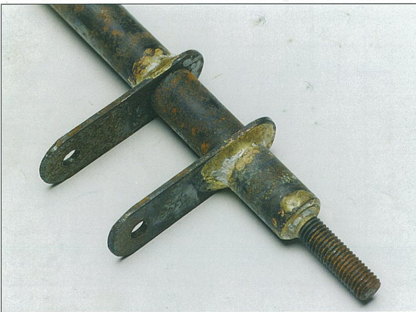
Fig. 5.17. The bottom of the steering column showing the bolt welded in place in the bottom of the tube, and the two track-rod plates in position. (Steve Williams)
