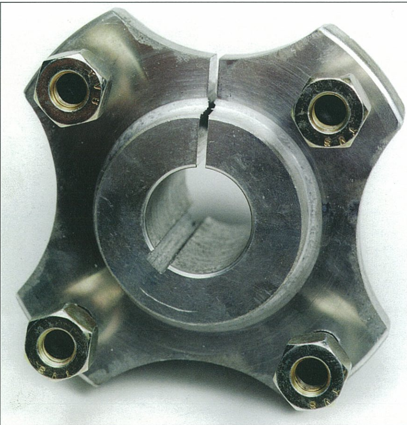
Fig. 7.3. Proprietary hubs can be obtained from go-kart specialist suppliers, but are likely to be quite expensive. (Steve Williams)
