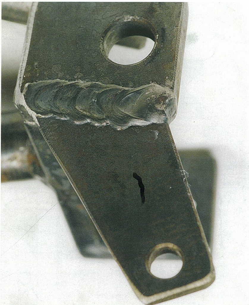
Fig. 5.8. A steering arm welded to the stub-axle carrier. (Steve Williams)
