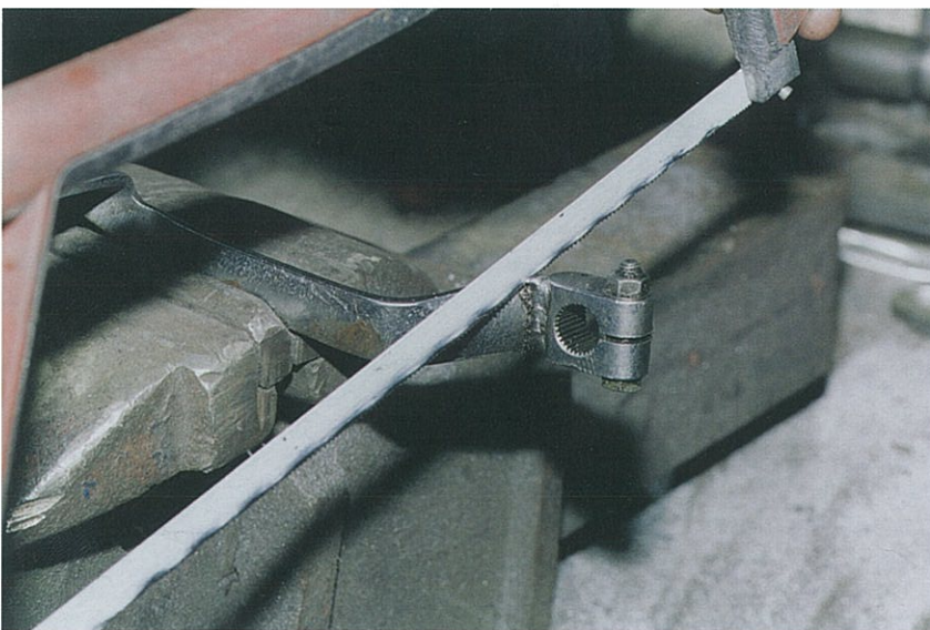
Fig. 8.12. Remove the boss from the pedal using a hacksaw. (Steve Williams)
