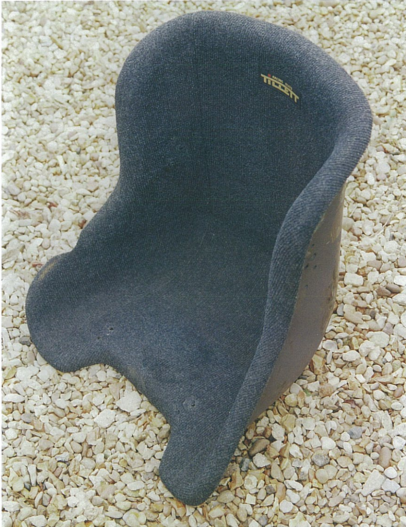
Fig. 3.6. This is a second-hand go-kart seat which cost £15, but the moulded seat from a stacking chair could be used and will only cost £1 to £2, if anything. (Steve Williams)
