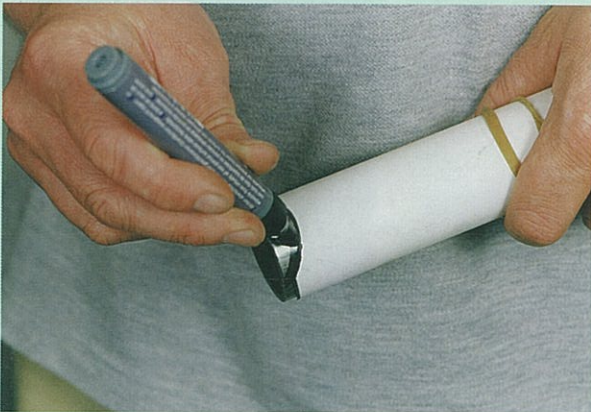
Slide the cardboard tube over the steel tube to be shaped and mark the fish-mouth outline on the steel tube with a felt-tip marker pen. (Steve Williams)
