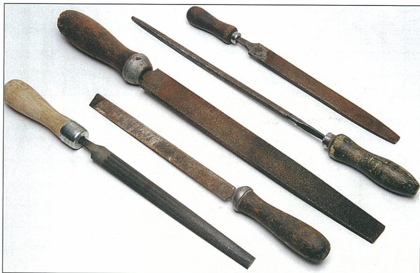
Fig. 2.10. A selection of files. It is essential that a correctly fitting handle is used at all times. (Steve Williams)
