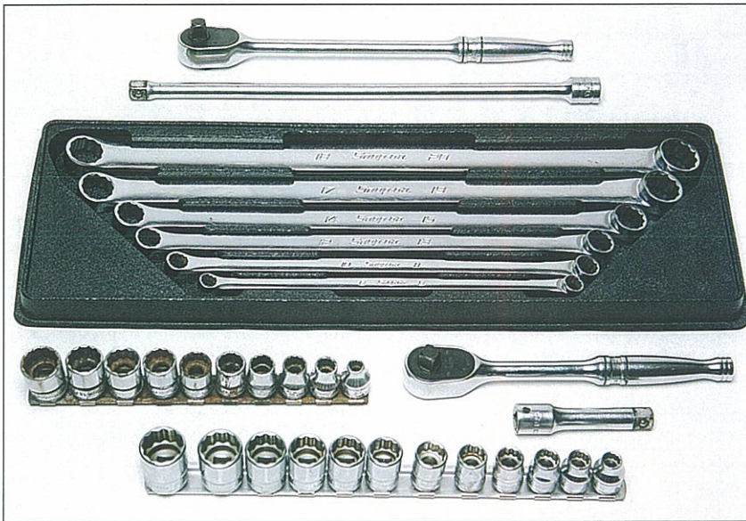
Fig. 2.1. A good quality set of sockets and spanners will last a lifetime. A selection of different lengths of socket-set extension is useful. Keeping your sockets on bars, as shown, will make it easier to select them for use and prevent them becoming lost. (Steve Williams)
