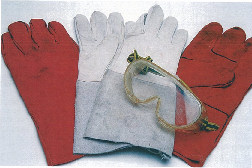
Fig. 2.13. Gauntlets and goggles. Essential for grinding and cutting operations. (Steve Williams)
