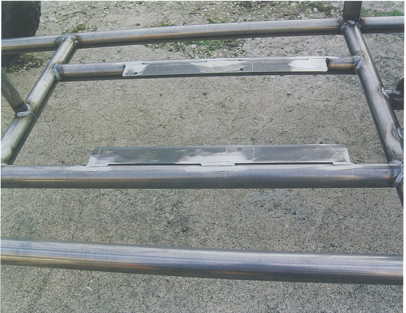
Fig. 4.18. Seat mounting plates welded in position. These have only 4 holes drilled for a non-adjustable seat. If you want the position of the seat to be adjustable, then you can drill a series of holes. (Steve Williams)
