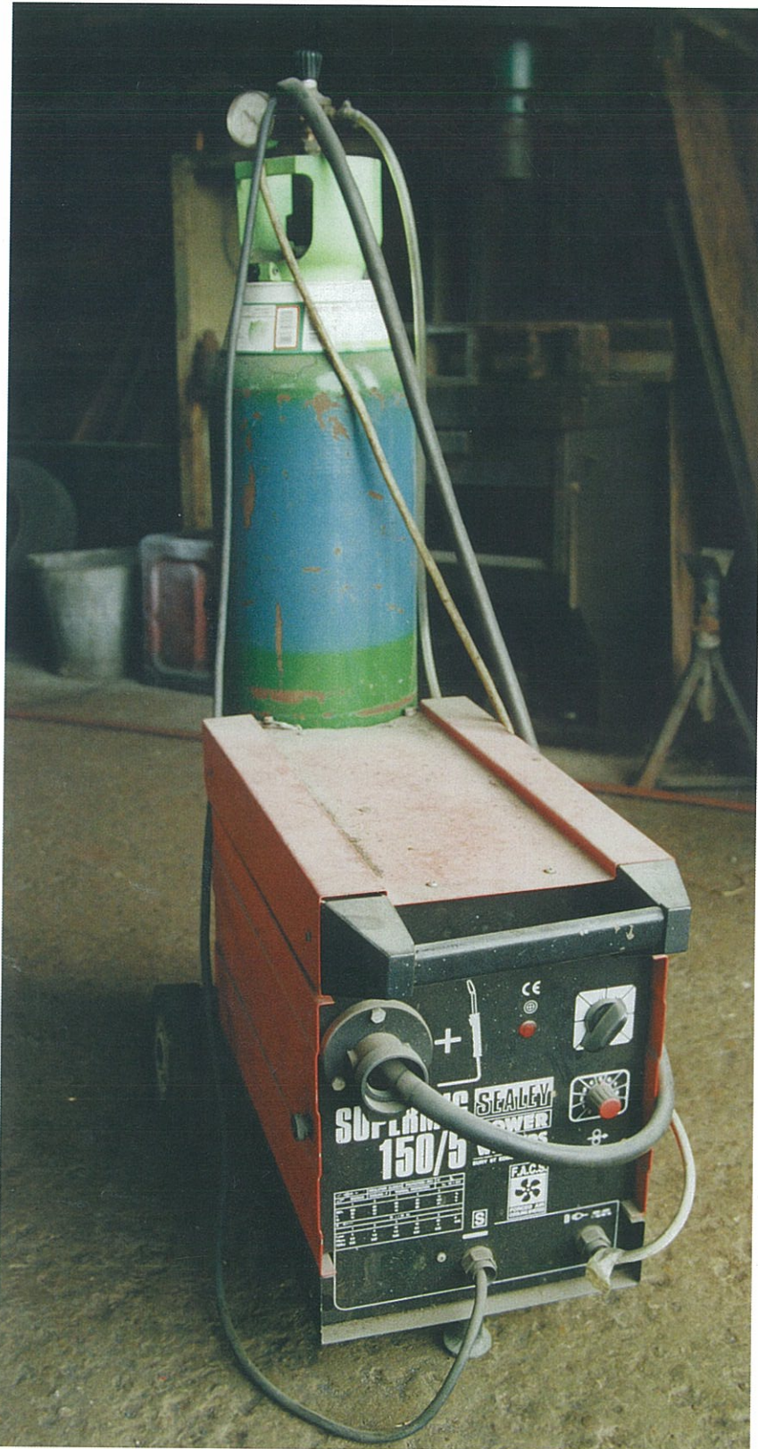
Fig. 1.3. A portable MIG welder. Remember you must wear a full-face shield to protect you from the ultraviolet light given off, and thick gloves should be used to stop your hands getting burnt. (Steve Williams)
