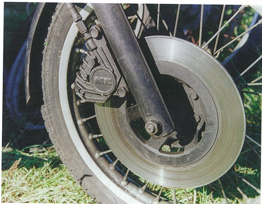
Fig. 3.5. A disc and caliper both in good order. The disc looks fairly new and you can see from the bright shiny surface finish that the bike was in use until recently. Beware of buying a donor bike that has been laid up for a while and has a rusty disc and, possibly, a seized caliper. (Steve Williams)
