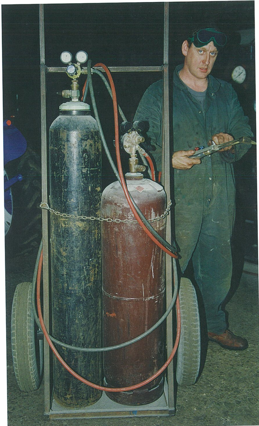
Fig. 1.1. Gas welding equipment. The taller cylinder contains oxygen, the shorter one acetylene. Suitable protective clothing, dark goggles or a mask and thick gloves should be worn when welding. (Steve Williams)
