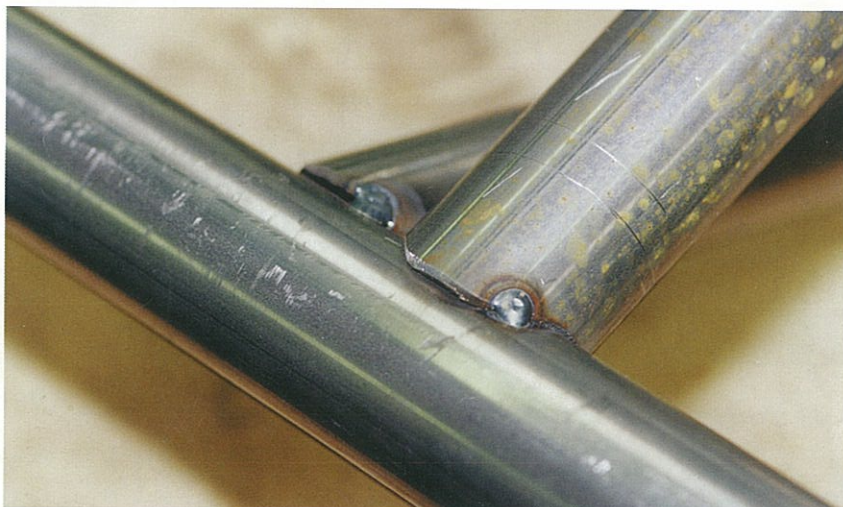
Left: Fig. 4.11. Main frame tube I tacked in position. Note the excellent fit produced by fish-mouthing the tubes. (Steve Williams)
