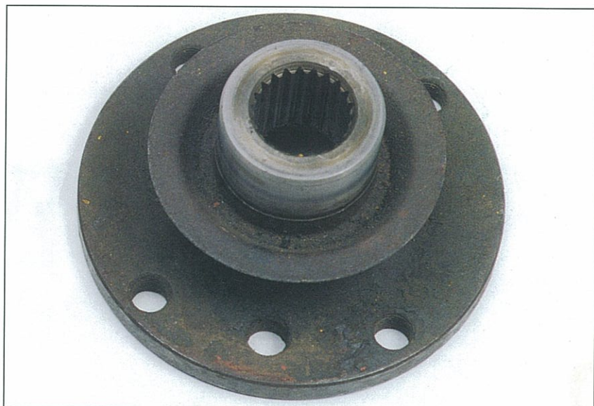
Fig. 3.9. A Ford differential flange, in this case from a Ford Capri, obtained for £2.50 from a scrapyard. (Steve Williams)
