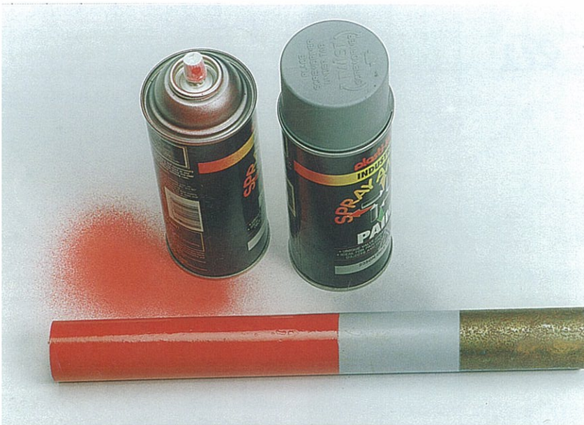
Fig. 1.4. Painting – two coats of grey primer and two coats of gloss paint will give a smart and durable finish which is easily touched up if damaged and, best of all, is cheap. (Steve Williams)
