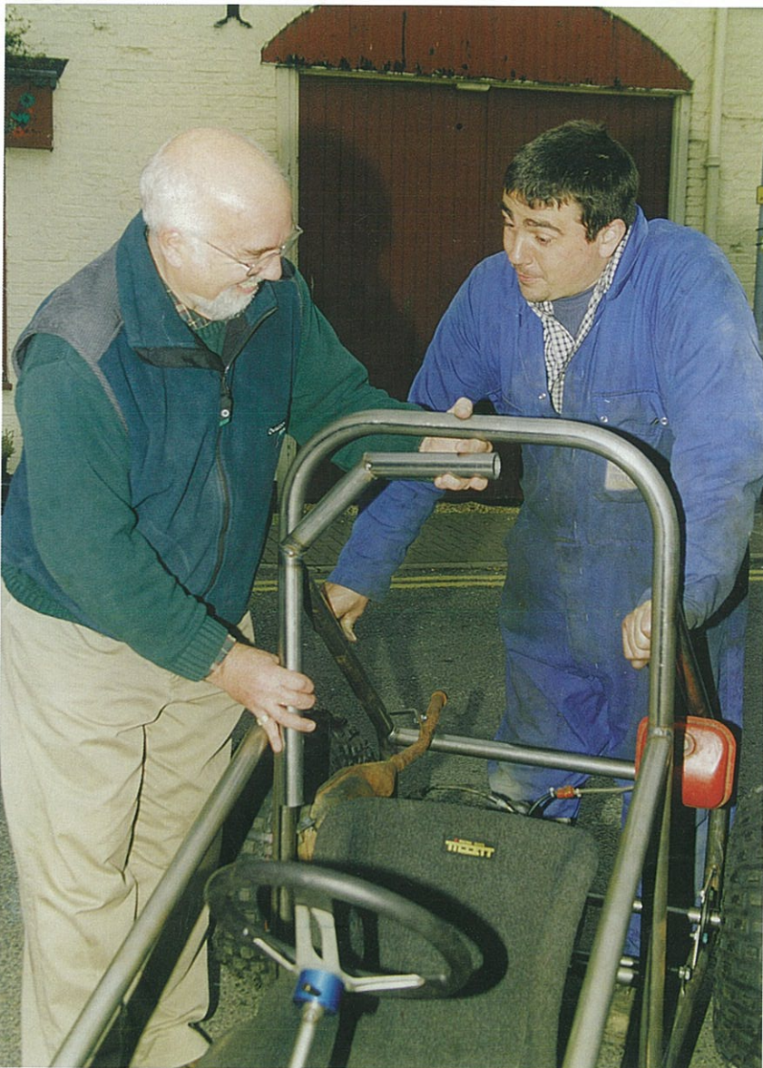
Left: Fig. 4.9. An alternative method for producing the roll bar if you don't have access to a tube bender is to fabricate from sections of tube cut at an angle. (Steve Williams)
