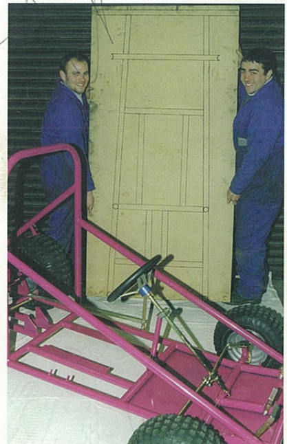
Fig. 4.6. The frame building board used for the original Buggy. Note that the frame tapers towards the front for purely cosmetic reasons. (Steve Williams)
