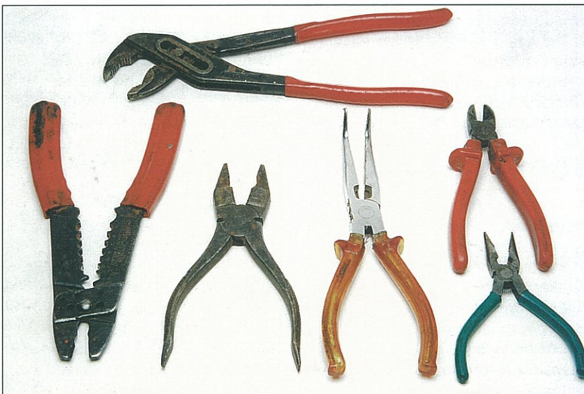
Fig. 2.3. A selection of pliers, including wire strippers and wire cutters. (Steve Williams)
