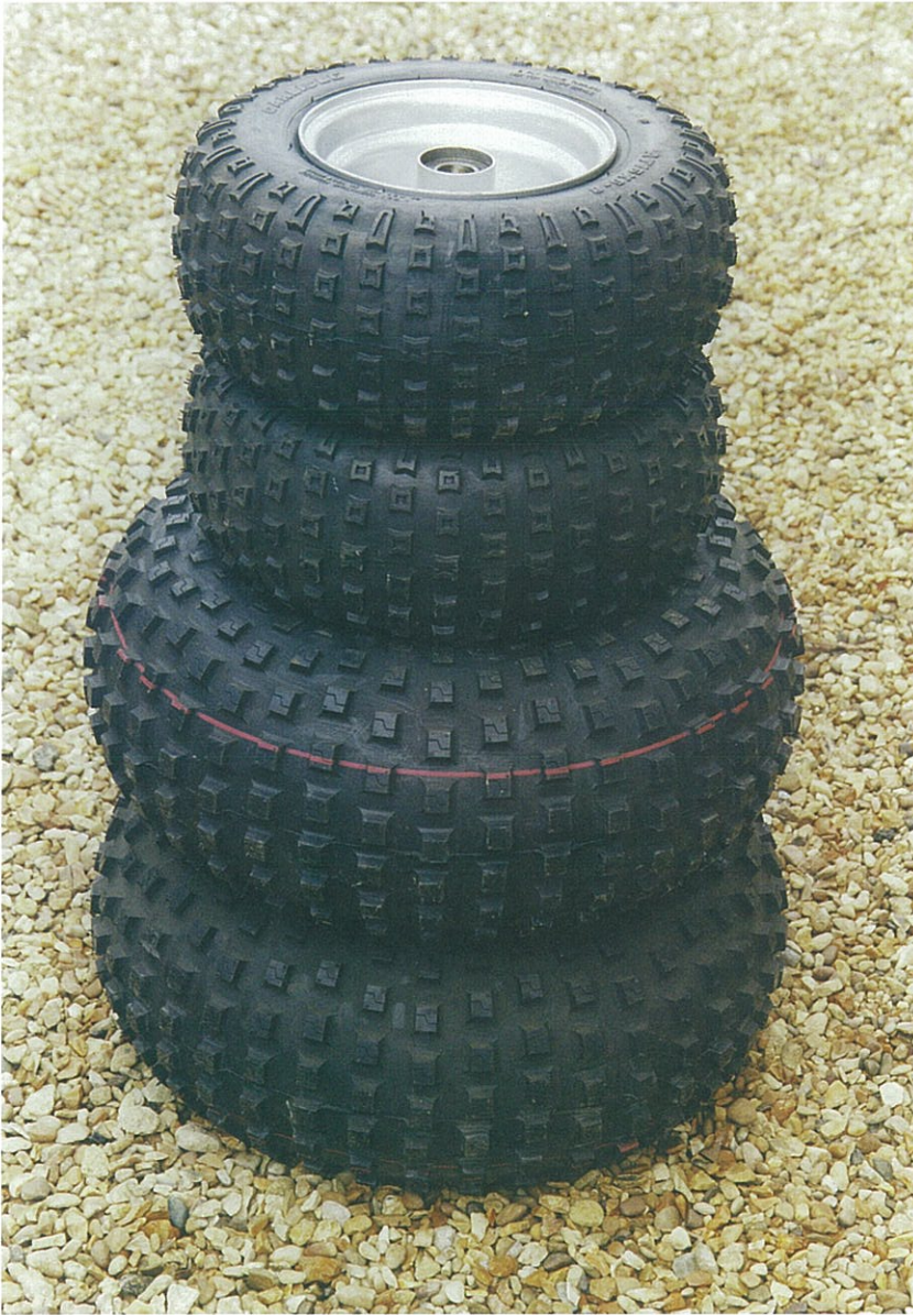
Fig. 3.10. These balloon tyres were sourced from a farm machinery factors and are usually used on quad bikes. The hubs have the same stud pattern as Mini wheels and come complete with bearings. (Steve Williams)
