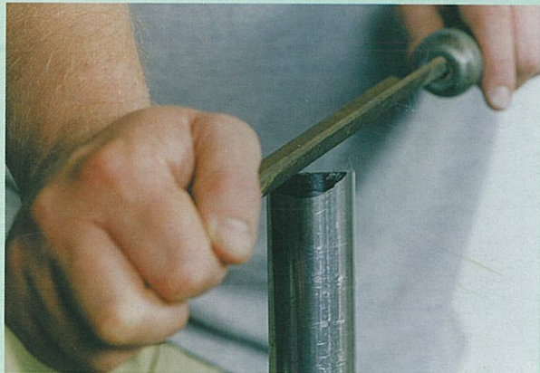
File the tube to shape using a half-round file. (Steve Williams)
