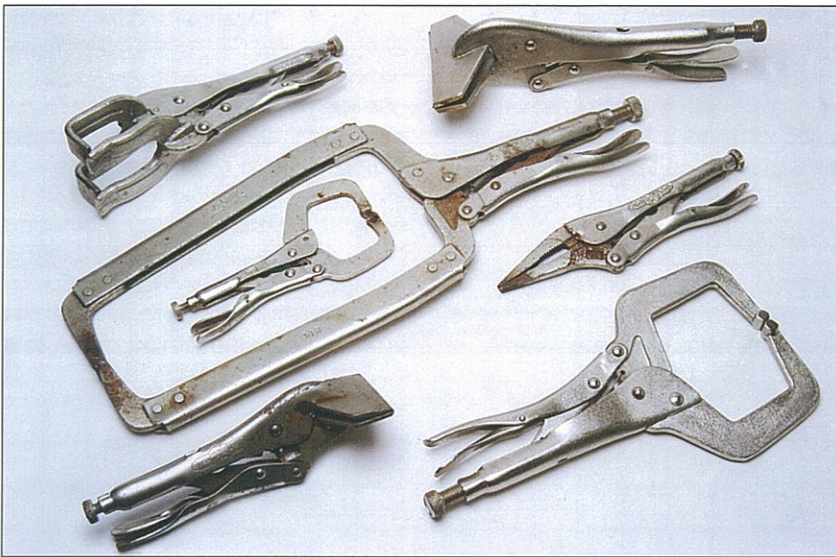
Fig. 2.11. A selection of self-grip clamps for holding metal items together when welding. (Steve Williams)
