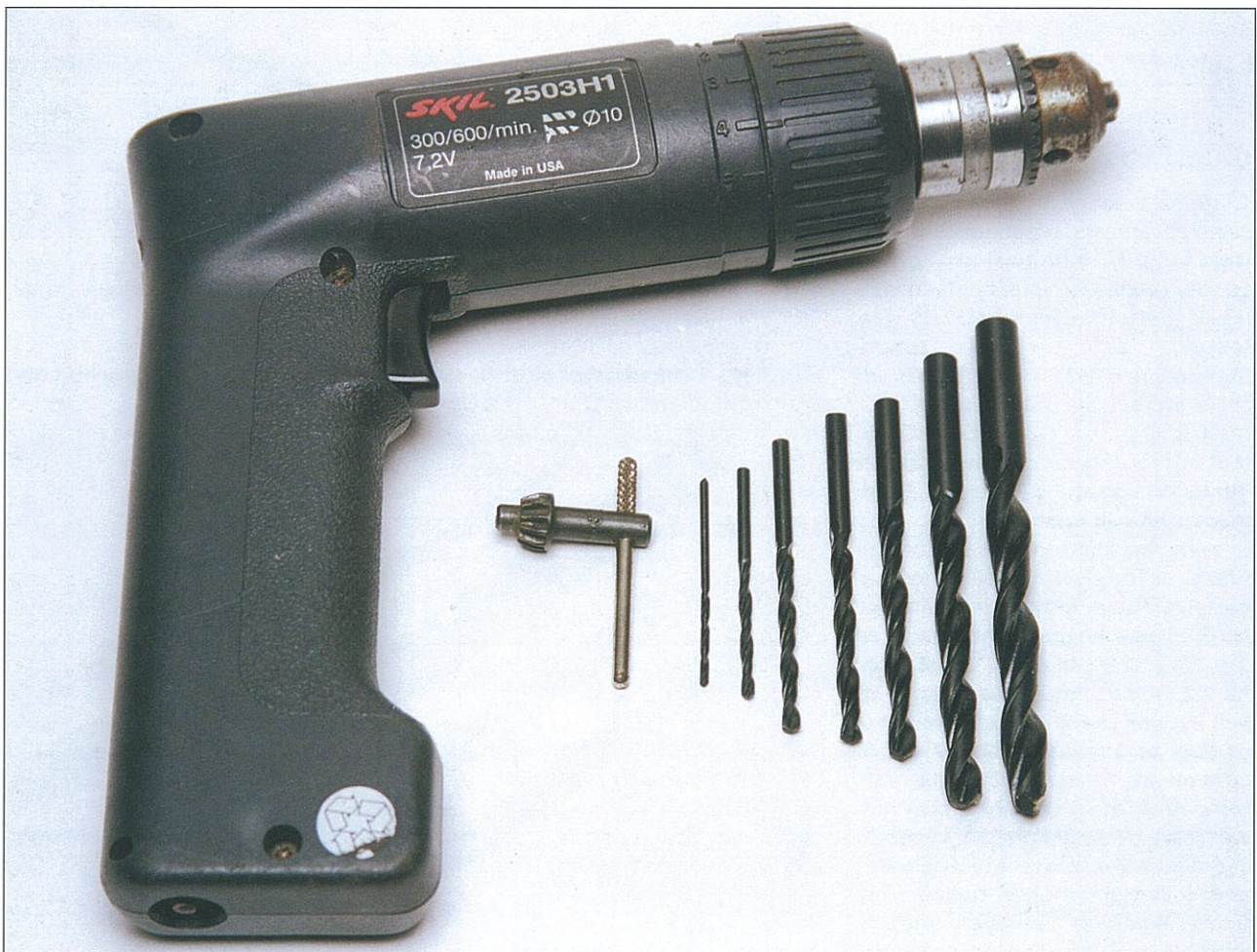
Fig. 2.12. A battery-operated rechargeable drill. Not essential if you have a mains-operated drill, but so light and compact to use. (Steve Williams)
