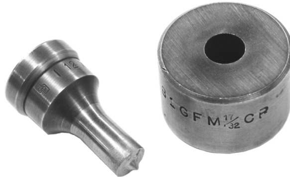
Figure 1 - Very high carbon steel punch and die.
