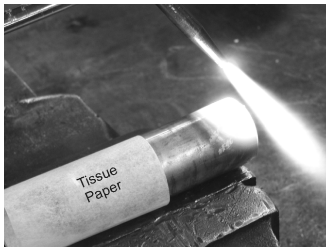
Figure 2 - Titanium pipe wrapped in tissue paper.
