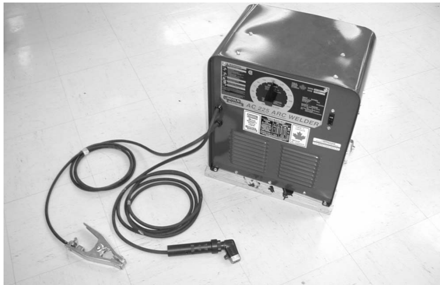
Figure 11 - AC transformer welding power source. (Courtesy Lincoln Electric)
