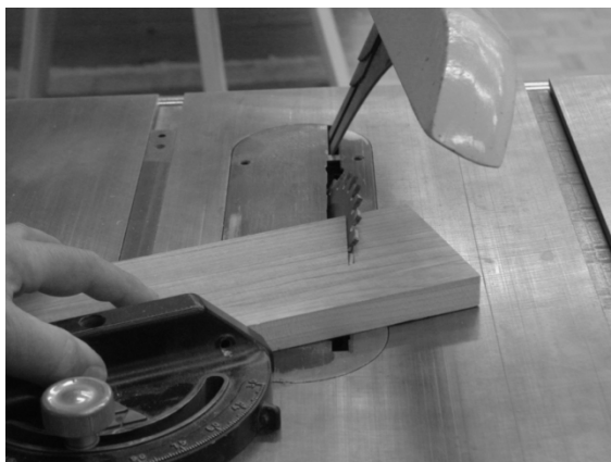
Figure 8 - Cutting a compound mitre.
