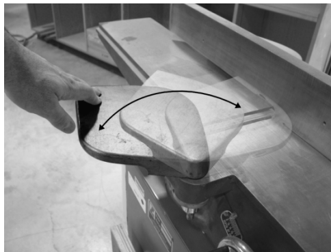
Figure 36 - Checking the guard for proper movement.
