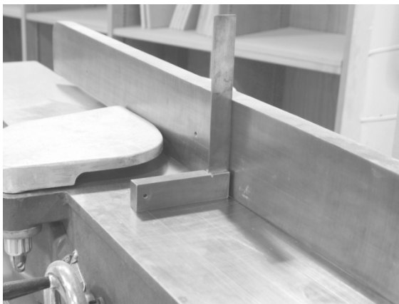
Figure 37 - Setting the fence square with the table.
