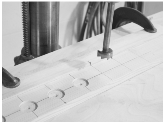
Figure 48 - Repetitive drilling with a drill press.
