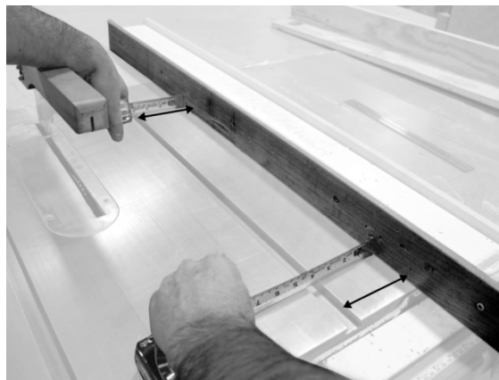
Figure 10 - Checking rip fence.
