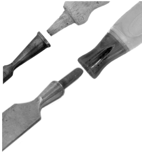
Figure 36 - Socket and tang connections for wood chisels.
