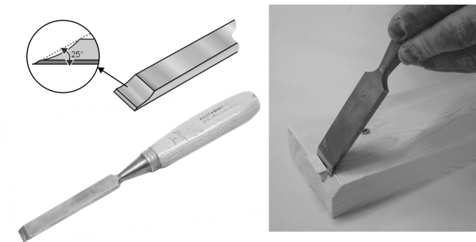
Figure 37 - Firmer chisel.
