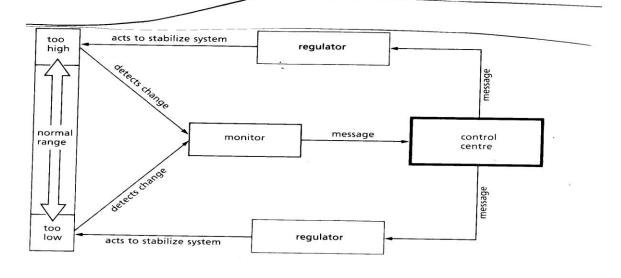
The Components of a Feedback System. Each component is differently coded. This pattern will be retained in the illustrations of feedback systems that follow.
